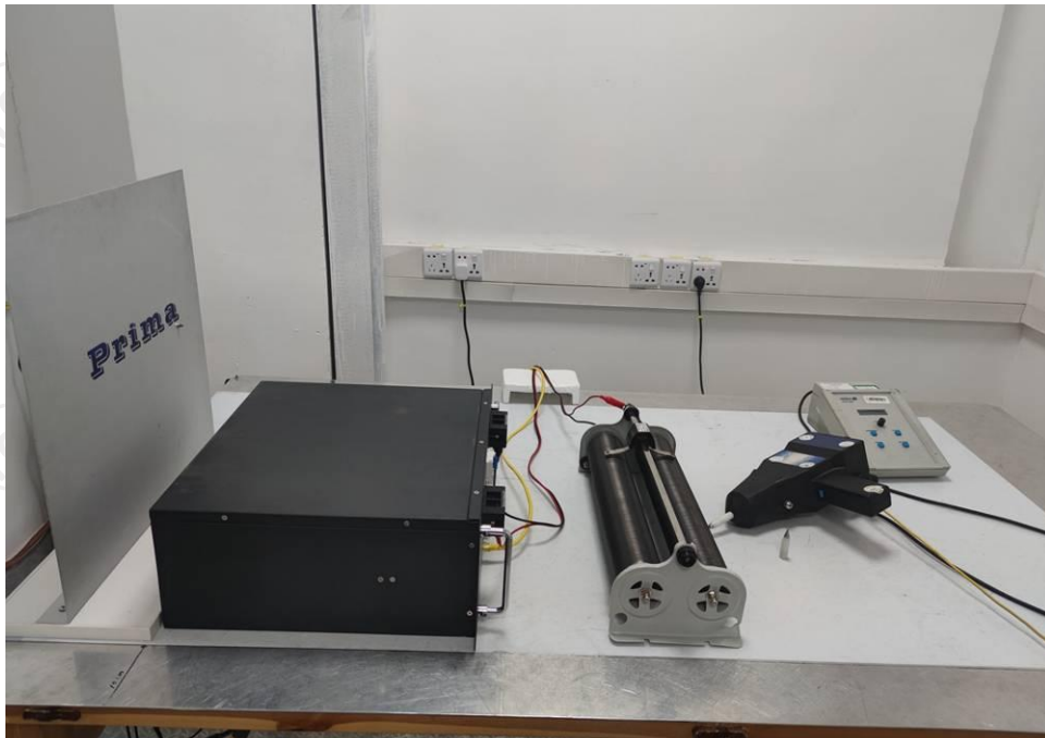
Electrostatic discharge immunity (ESD) test view
